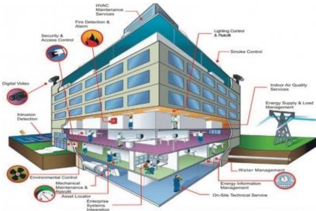
Figure 4 Building Management System (BMS) Error! Reference source not found.
